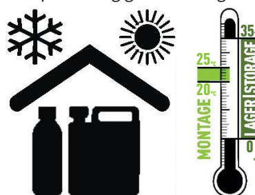
Abb. 7: Storage and processing of the sleeve foam.
