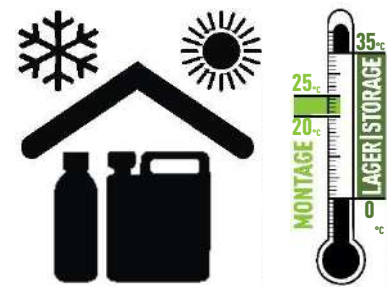
Abb. 7: Storage and processing of the sleeve foam.
